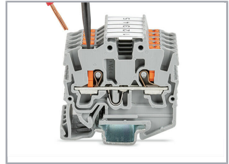
Insert fine-stranded conductors via operating tool.
