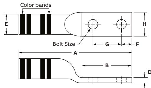
**Aluminum lugs — narrow-tongue, long-barrel, two-hole**
