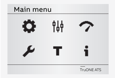
Fig. 4.6 By pressing Enter-key (3) you will move to the main menu page of Operation, Parameters, Measurements, Settings, Test and About, see the table below for the selections. You can move in menu or choose parameter values by Up and Down -keys (2) and by Enter-key (3) you can accept function and enter a new menu page. By Esc-key (1) you can go back in menu.
