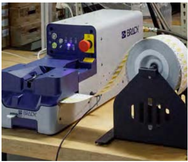
Feed printed PermaSleeve roll into the BSP45 Applicator
