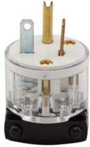
Eaton Arrow Hart safety grip hospital grade straight blade plug, #18-12 AWG, 20A, Industrial, Flush, 125V, Back and side, Clear, Brass, Polycarbonate with thermoplastic housing, 5-20P, Two-pole, three-wire, grounding, Screw, 0.25-0.69" dia, Core pack
