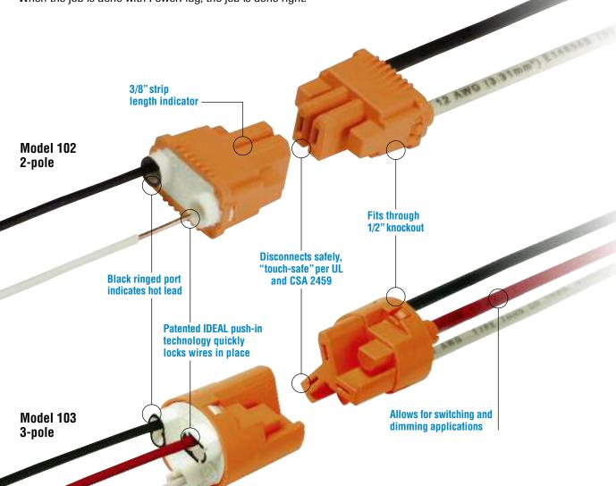
• 3-pole disconnect allows for one-connector installation of many of today's energy-saving lighting configurations, such as fixtures with dual or electronic ballasts
