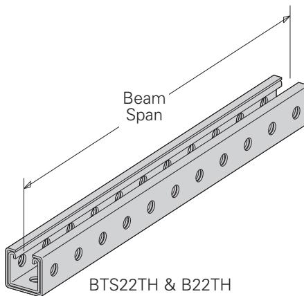
\*Based on simple beam condition using an allowable design stress of 25,000 psi (172 MPa) with adequate lateral bracing (see page 12 for further explanation). To determine concentrated load capacity at mid span, multiply uniform load by 0.5 and corresponding deflection by 0.8.
