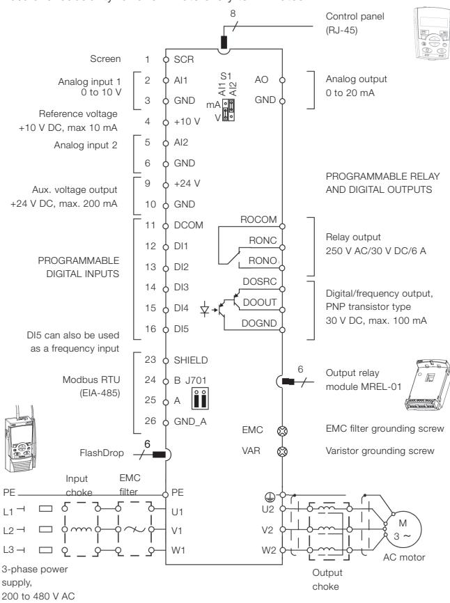
Note: For 1-phase power supply, connect power to U1/L and V1/N terminals.
