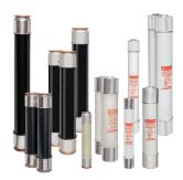
Mersen fuses for the protection of transformers and distribution lines deliver overload and short circuit protection. These current-limiting fuses will melt at current that can be as low as 1.7 times the fuse current ratings up to its maximum interrupting rating. These fuses are designed to withstand the transformer magnetizing inrush current. They have 2 (size C), 3 (size D) and 4 (size E) inch diameter barrels with ferrules and are mounted in spring reinforced clips.
