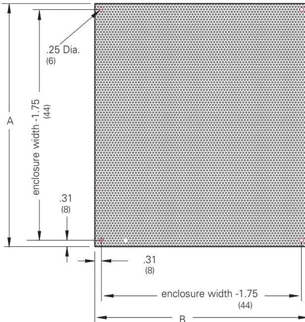
JIC perforated panels can be installed in all types of JIC Enclosures, and are intended for mounting lightweight components without drilling and tapping.
