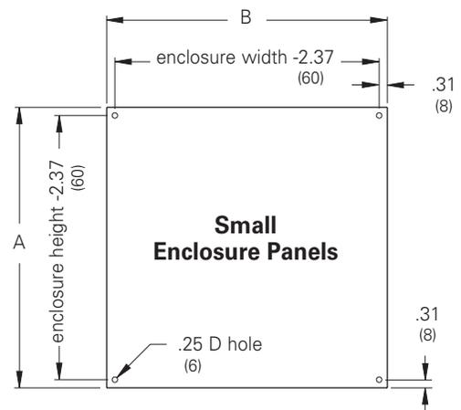
Small Enclosure panels can be installed in Small Type 3R RHC and Small Type 1 Enclosures. Panels are only available in steel, and have a white powder finish.
