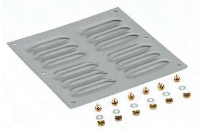
Excellent for providing ventilation in enclosures where external conditions or internal components may cause excessive amount of heat or moisture. Designed to be used with B-Line series Filter Kits using the same cut-out and mounting hole configurations. Louver Plate Kits include all of the necessary hardware and instructions for field installation. Plates are constructed from 16 gauge steel and have an ANSI 61 gray polyester powder finish.
