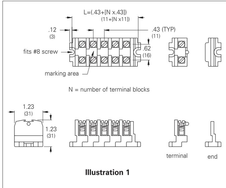
**Heavy-Duty Flat Base** terminal blocks are rated at 600 VAC, 90 Amps. Terminal lugs are plated copper and have tubular screw contacts. Terminal wire range is from #18 through #4 AWG. Each terminal block top has a painted marking area intended for circuit designation. These blocks are designed to stack in combination with both Heavy-Duty and/or Medium-Duty Flat Base type terminals. One Flat Base Terminal End and hardware is required to terminate a stack of blocks (order separately).
