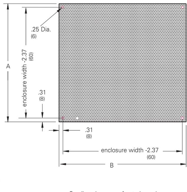
Small enclosure perforated panels can be installed in small Type 3R RHC, and small Type 1 Enclosures, and are intended for mounting lightweight components without drilling and tapping.
