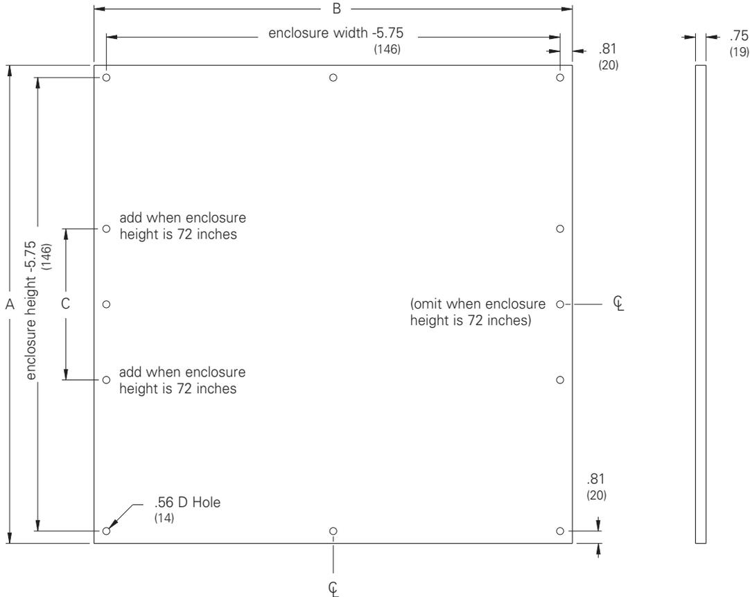
Large Flanged Panels can be installed in Floor Standing Type 4X, Type 4 and Type 12 Enclosures. Handle Kits are furnished with each panel. Steel panels have a white powder paint finish. Stainless steel and aluminum panels have a smooth brushed finish on one side and protected with PVC film.
