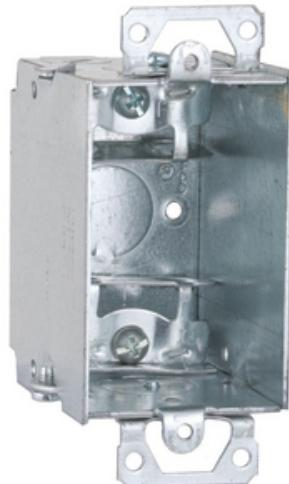
3 in. x 2 in. Switch Box, Gangable, 2-1/2 in. Deep One 1/2 in. KO & AC/MC/Flex Clamps, Plaster Ears
