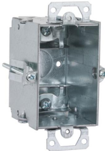
3 in. x 2 in. Switch Box, Gangable, 2-1/2 in. Deep with One 1/2 in. KO & AC/MC/Flex Clamps, Grintite, Old Work
