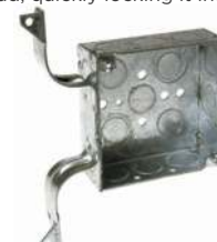
"W" Bracket Positions box away from side of stud to clear the trim molding of a door frame.
