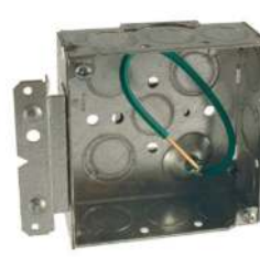
"H" Bracket Narrow bracket allows side-by-side mounting on stud. Positioning tabs locate box perfect distance from stud. V notch centers box. Dimples protect flush drywall installation.
