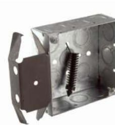
Box-Loc® "MS" Bracket Positions box on either side of stud. BOX-LOC® (MS) Bracket Box is a snap to install. Place the bracket on the open side of the stud first. Slots in the bracket engage the lip of the stud and actually crimp it as you press the bracket on the stud. Barbed hooks dig into the flat side of the stud, quickly locking it into place.
