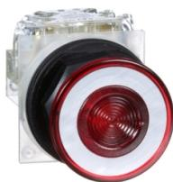
30mm Push Button, Type SK, push pull operator, red mushroom cap, 1 NO and 1 NC
