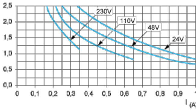
AC14 control of small electromagnetic loads  $\leq 72$  VA, make:  $\cos \phi = 0.3$ , break:  $\cos \phi = 0.3$ .
