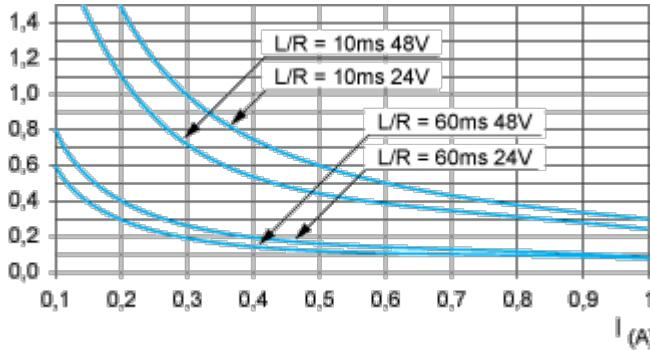
DC13 switching electromagnets,  $L/R \leq 2 \times (U_e \times I_e)$  in ms,  $U_e$ : rated operational voltage,  $I_e$ : rated operational current (with a protective diode on the load, DC12 curves must be used with a coefficient of 0.9 applied to the number in millions of operating cycles)**AC Loads**
