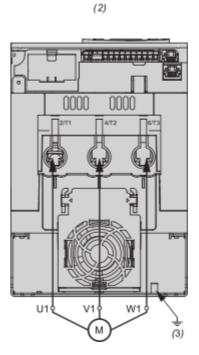
Use class C cables for the power connections.
