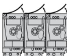
Remove the protective cover from the top of the drive.
