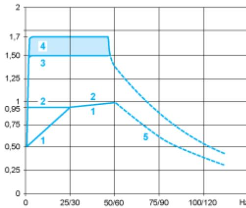
1 : Self-cooled motor: continuous useful torque (1)
