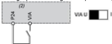
Analog input VIA configured as negative logic input ("Sink" position)
