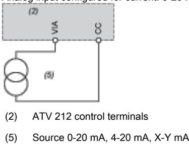
Analog input VIA configured as positive logic input ("Source" position)
