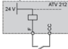
"PLC" position with PLC transistor outputs
