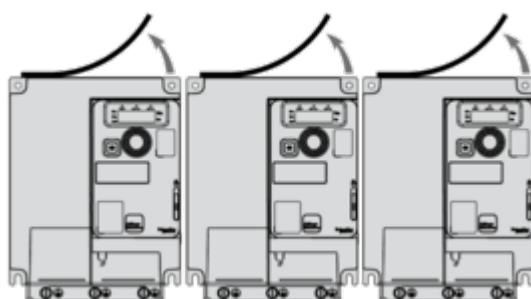
**Mounting Type C: Individual, Ventilation Cover Removed**
