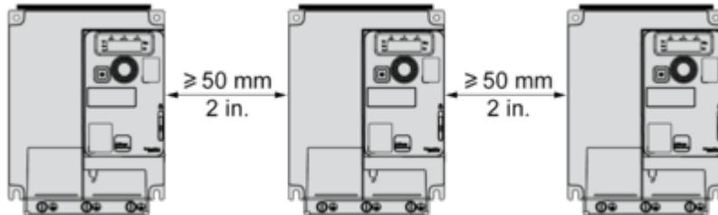
Only Possible at Ambient Temperature Less or Equal to 50 °C (122 °F)
