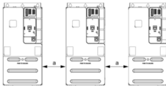
$a \geq 50 \text{ mm (1.97 in.)}$  from  $50\ldots60^{\circ}\text{C}$ , no restriction below  $50^{\circ}\text{C}$
