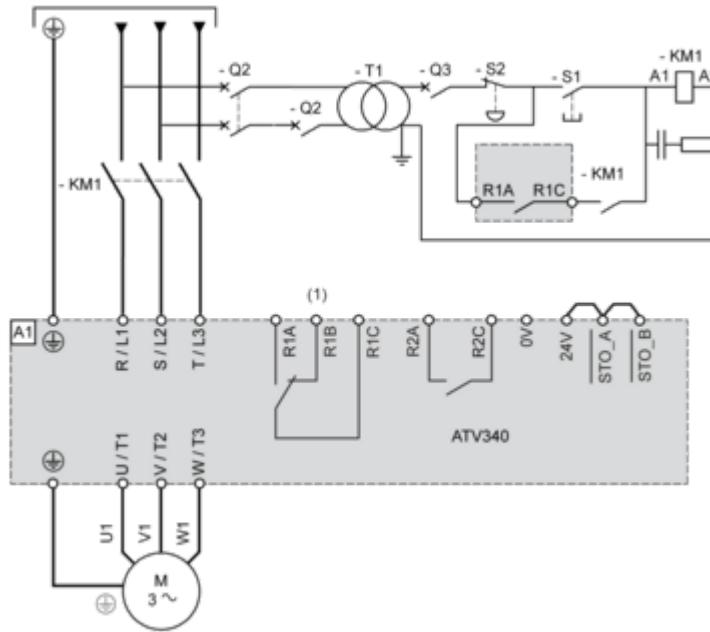
(1) : Use relay output R1 set to operating state Fault to switch Off the product once an error is detected.
