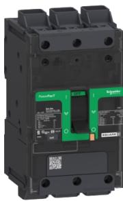
Circuit breaker, PowerPact B, 30A, 3 pole, 600Y/347VAC, 18kA, lugs, thermal magnetic, 80%, control wire ON end
