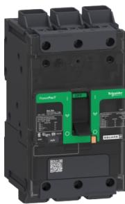
Circuit breaker, PowerPact B, 50A, 3 pole, 600Y/347VAC, 18kA, lugs, thermal magnetic, 80%, control wire ON end
