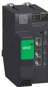
standalone processor, Modicon M580, 16MB, 125 Ethernet devices, 8 local IO racks of 4096 digital, 1024 analog
