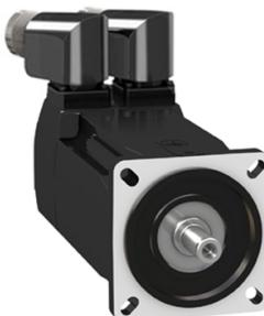
**servo motor BMH, Lexium 32, 1.2Nm, 8000rpm, untapped shaft, without brake, IP54, 16 multturn encoder**
