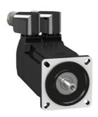
servo motor BMH, Lexium 32, 2.5Nm, 8000rpm, untapped shaft, without brake, IP54, 16bit encoder, 3 phases
