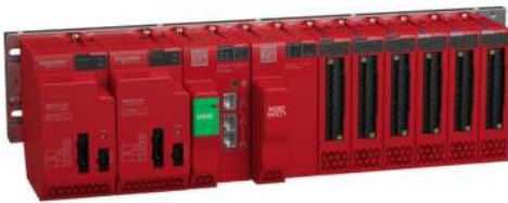
Modicon Safety configuration with Modicon X80 Safety modules only with removable terminal blocks
