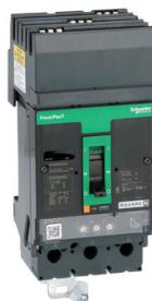
Circuit breaker, PowerPact J, 250A, 3 pole, 600VAC, 18kA, I-Line, Micrologic 3.2S, 80%, ABC
