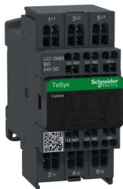
IEC contactor, TeSys Deca, nonreversing, 9A, 5HP at 480VAC, 3 phase, 3 pole, 3 NO, 24VDC coil, open style
