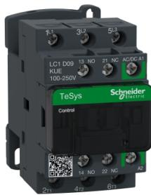
IEC contactor, TeSys Deca, nonreversing, 9A, 5HP at 480VAC, up to 100kA SCCR, 3 phase, 3 NO, 100/250VAC/VDC coil, open
