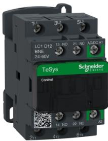
IEC contactor, TeSys Deca, nonreversing, 12A, 7.5HP at 480VAC, up to 100kA SCCR, 3 phase, 3 NO, 24/60VAC/VDC coil
