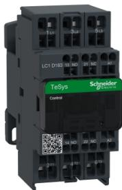
IEC contactor, TeSys Deca, nonreversing, 18A, 10HP at 480VAC, 3 phase, 3 pole, 3 NO, 24VAC 50/60Hz coil, open style
