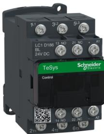
IEC contactor, TeSys Deca, nonreversing, 18A, 10HP at 480VAC, 3 phase, 3 pole, 3 NO, low consumption 24VDC coil, open style
