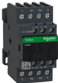
IEC contactor, TeSys Deca, nonreversing, 40A resistive, 4 pole, 2 NO and 2 NC, 120VAC 50/60Hz coil, open style
