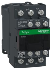
IEC contactor, TeSys Deca, nonreversing, 32A, 20HP at 480VAC, 3 phase, 3 pole, 3 NO, 24VDC coil, open style
