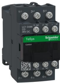
IEC contactor, TeSys Deca, nonreversing, 38A, 20HP at 480VAC, 3 phase, 3 pole, 3 NO, 36VDC coil, open style
