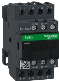
IEC contactor, TeSys Deca, nonreversing, 25A resistive, 4 pole, 4 NO, 230VAC 50/60Hz coil, open style
