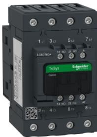
IEC contactor, TeSys Deca, nonreversing, 60A resistive, 4 pole, 4 NO, 240VAC 50/60Hz coil, open style
