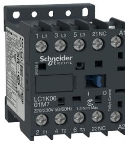
Contactor, TeSys K, 3P, AC-3, 1t or eq to 440V 6A, 1 NC aux., 24VAC coil
