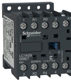
Contactor, TeSys K, 4P, 2 NO + 2 NC, AC-1,  $I_t$  or eq to 440V 10A, 24VAC coil
