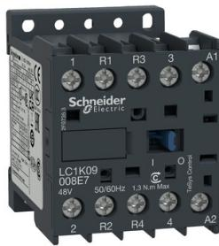
Contactor, TeSys K, 4P, 2 NO + 2 NC, AC-1,  $I_t$  or eq to 440V 10A, 120VAC coil
