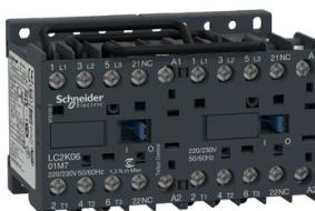
Reversing contactor, TeSys K, 3P, AC-3, It or eq to 440V 12 A, 1 NC, 230 to 240VAC
