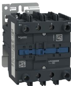
IEC contactor, TeSys Deca, nonreversing, 125A resistive, 4 pole, 2 NO and 2 NC, 24VDC coil, open style
