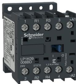
Contactor, TeSys K, 4P, 2 NO + 2 NC, AC-1,  $I_t$  or eq to 440V, 20A, 24VDC coil
