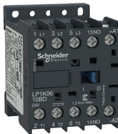
Contactor, TeSys K, 3P, AC-3, 1t or eq to 440V, 9A, 1 NO aux, 110VDC coil
