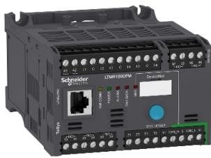
**Motor controller, TeSys T, Motor Management, DeviceNet, 6 logic inputs, 3 relay logic outputs, 5 to 100A, 100 to 240VAC**
